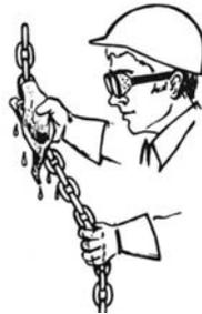
2 Hang chain vertically, if practical, for preliminary inspection. Measure reach accurately (bearing point of master link to bearing point of hook). Check this length against reach shown on tag. If present length is greater than that shown on tag, there is a possibility that the sling has been subjected to overloading or excessive wear.
